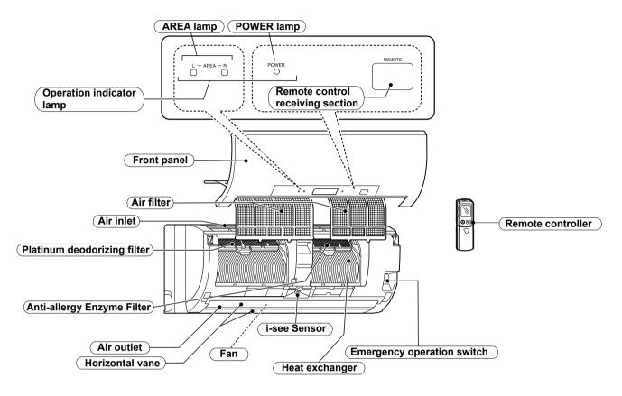
AREA lamp indicates AREA setting In AREA setting, the horizontal air flow direction changes automatically according to the detection of i-see Sensor which detects the floor/ wall
